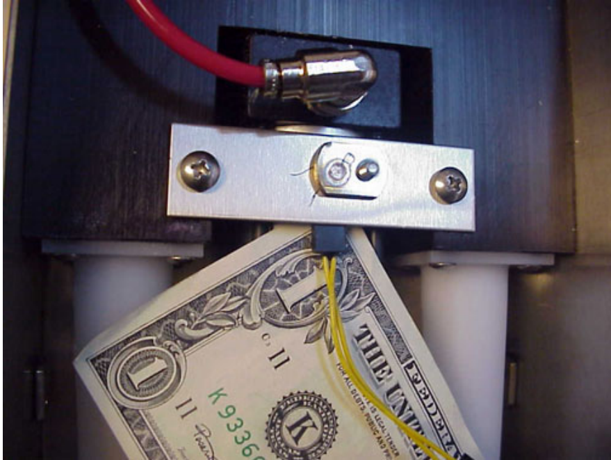
Figure 4: checking for space between the switch and the cylinder
