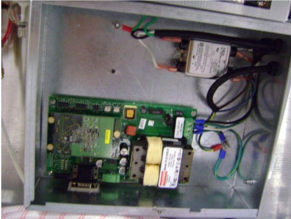
Figure 1 – New LonWorks software board. Note that this new board is green
