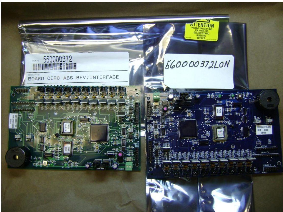
Figure 2: ABS Beverage Interface board. The blue board on the right (CCP# 121284) is compatible with the LonWorks Gateway
