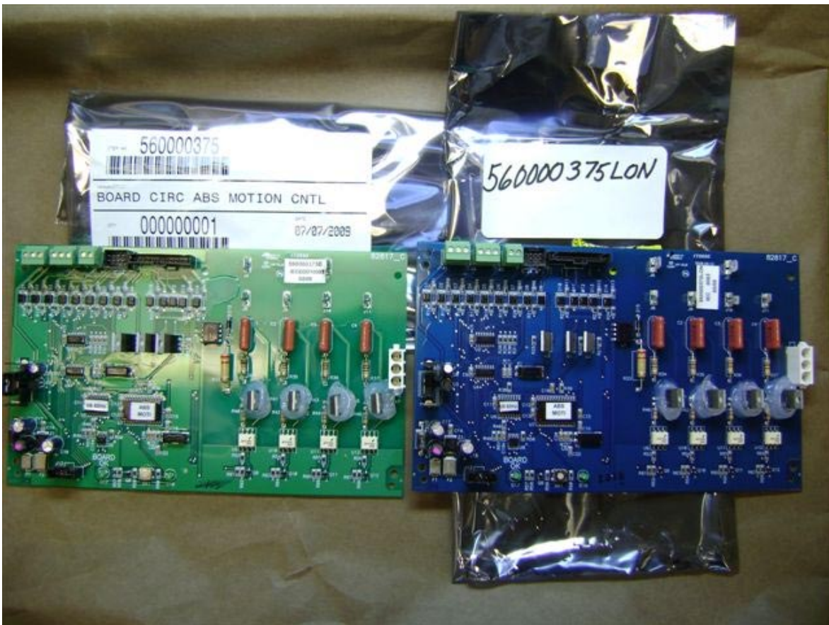
Figure 3: ABS Motion Control Board. The blue board on the right (CCP# 121285) is compatible with the LonWorks Gateway
