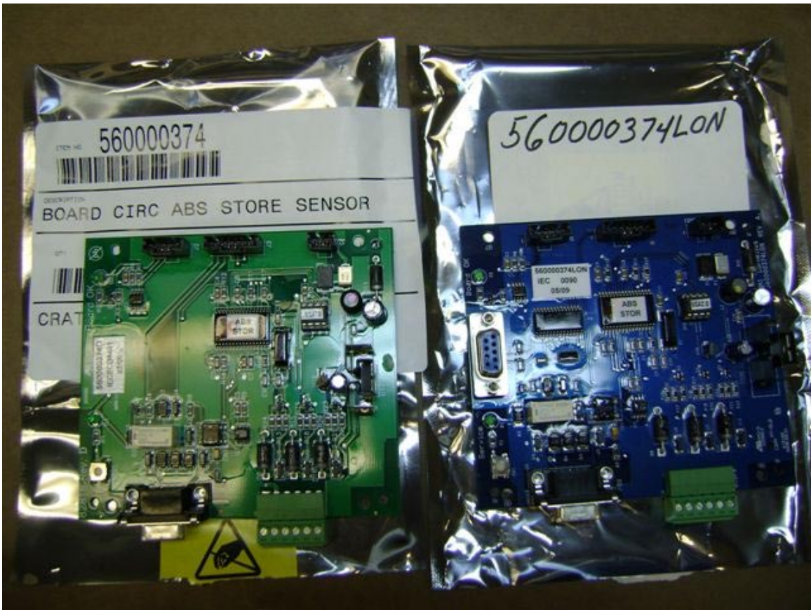
Figure 2: ABS Store Sensor Board. The blue board on the right (CCP# 121286) is compatible with the LonWorks Gateway
